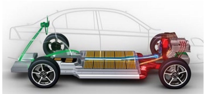
Figure 3. The CODA Vehicle Features an Air-Controlled Active Thermal Management System [6]
