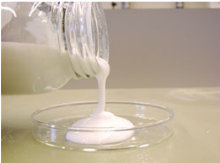
Figure 5. CryoSolPlus Material Could Enhance the Heat Absorbing Ability of EV Battery Liquid Cooling Systems [11]
