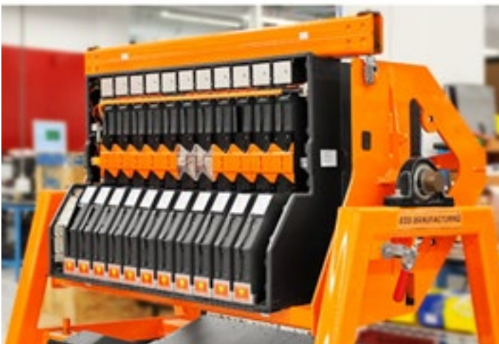
Figure 1. Under-Construction Lithium-Ion Battery Pack for Use in a Tesla Roadster [2]
